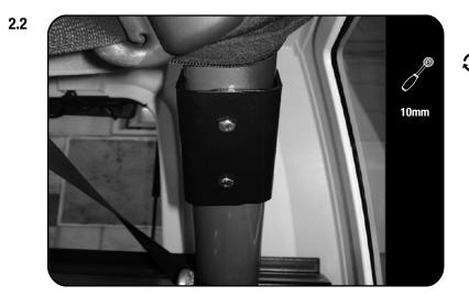
Locate the two threaded holes on the underside of the roll bar and fasten the two halves of the Roll Bar Clamps (Items 3 & 4) to the roll bar using M6 x 19 x 1SS Flat Washers and M6 x 20 Hex Bolts (Items 7 & 10). Place the Outer Roll Bar Clamp (Item 3) first, followed by the Inner Roll Bar Clamp (Item 4).
