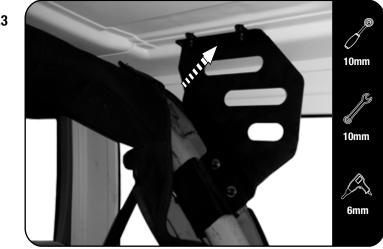
Loosely attach the Rear Support Arms (Item 1) to the outside of the Roll Bar Clamps using M6 x 20 Hex Bolts, M6 x 19 x 1SS Flat Washers and M6 Nyloc Nuts (Items 7, 10 & 11). Make sure the foot faces the inside of the vehicle as shown.
